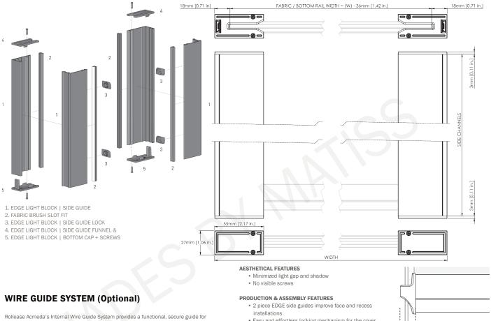
the S45 Roller Shade series, aiding and controlling a shade from unwanted movement.
